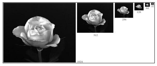
To see the effects resulting from the reduction in the number of samples, we bring all the subsampled images up to size 1024×1024 by row and column pixel replication. The resulted images are shown in the following Figure.
