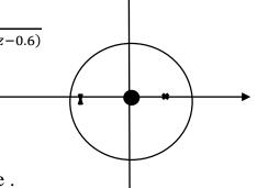
**EXAMPLE:** Find poles and zeros for  $x(z) = \frac{z}{z - \frac{1}{2}} + \frac{z}{z + \frac{1}{3}}$
